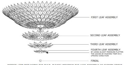
NOTICE: FOR REPLACING THE BULB, PLEASE UNSCREW THE LEAF ASSEMBLY AS SHOWN ABOVE.
