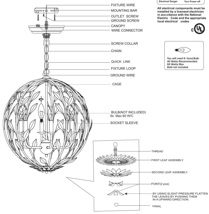
ASSEMBLE THESE PARTS TO THE BOTTOM
