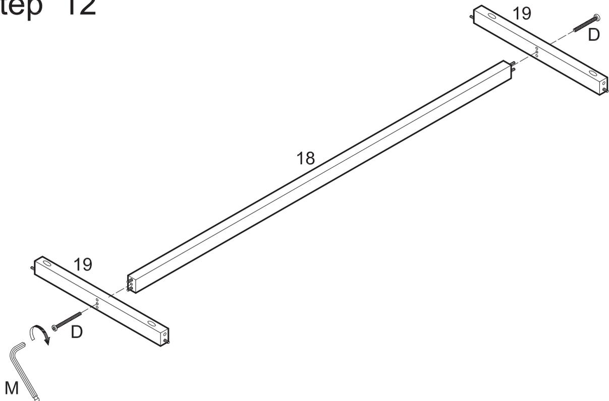
Attach crossbars (19) to crossbar (18) using bolts (D). Tighten bolts (D) with wrench (M).
