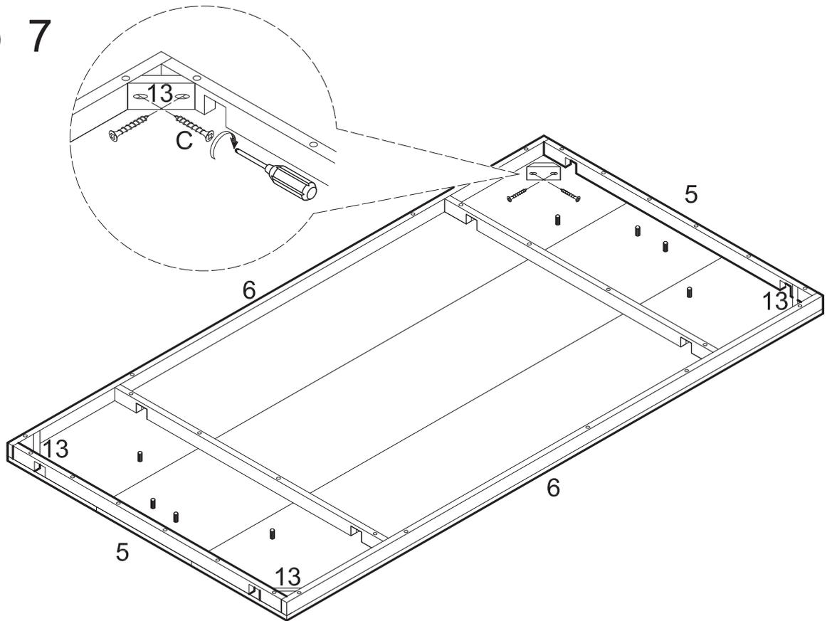
Attach corner blocks (13) to slats (5,6) using screws (C).
