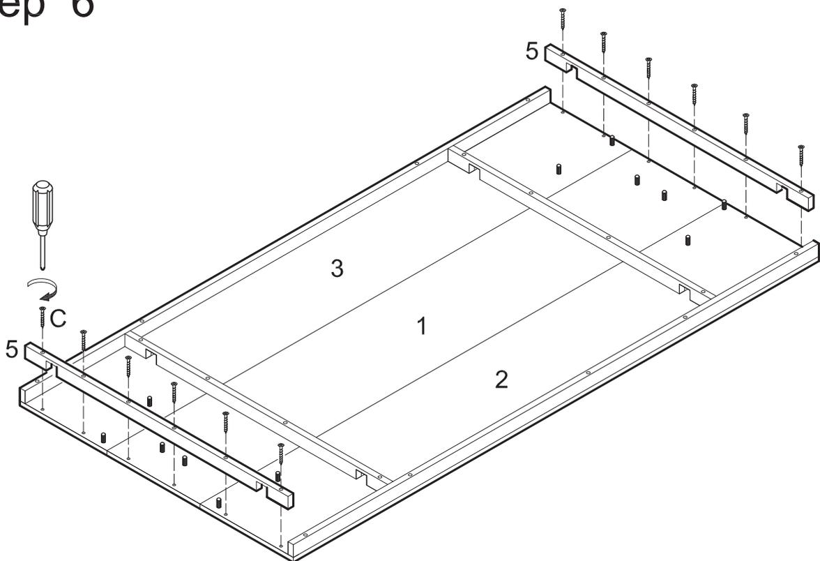
Attach slats (5) to table top pieces (1,2,3) using screws (C).
