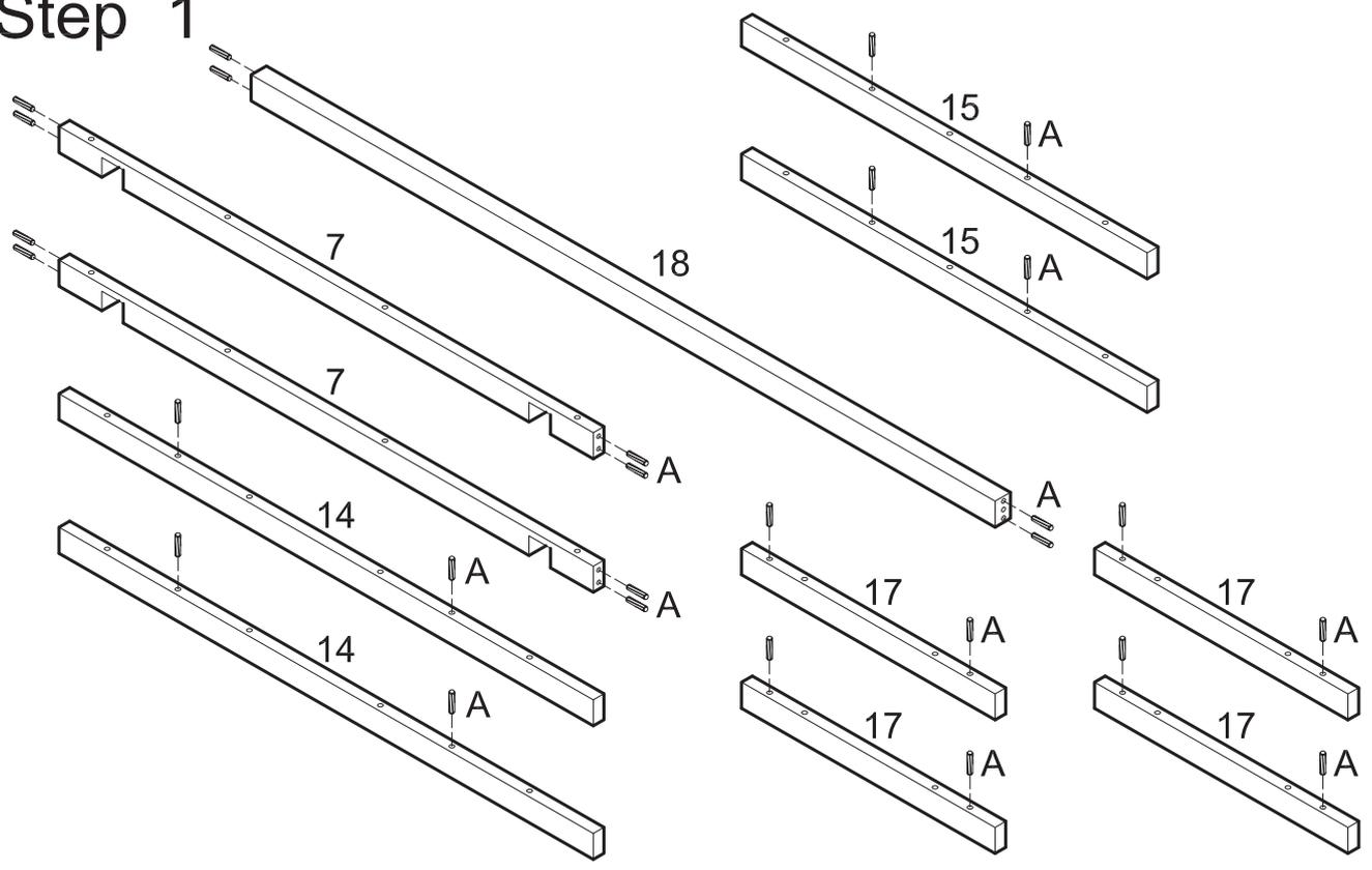
Insert dowels (A) into slats (7,14,15,17) and crossbar (18) as shown above.
