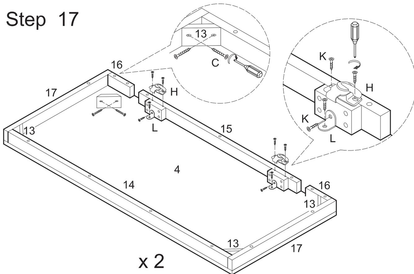
Attach corner blocks (13) to slats (14,16,17) using screws (C). Attach table locks (H) and brackets (L) to slat (15) using screws (K). Repeat this step for second leaf (4).
