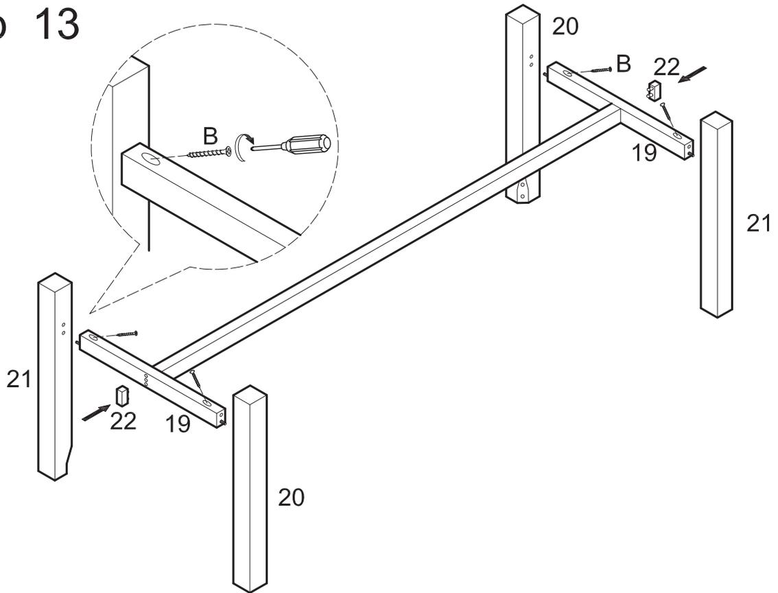
Attach crossbars (19) to legs (20,21) using screws (B). Attach end caps (22) to crossbars (19) using dowels as guides.
