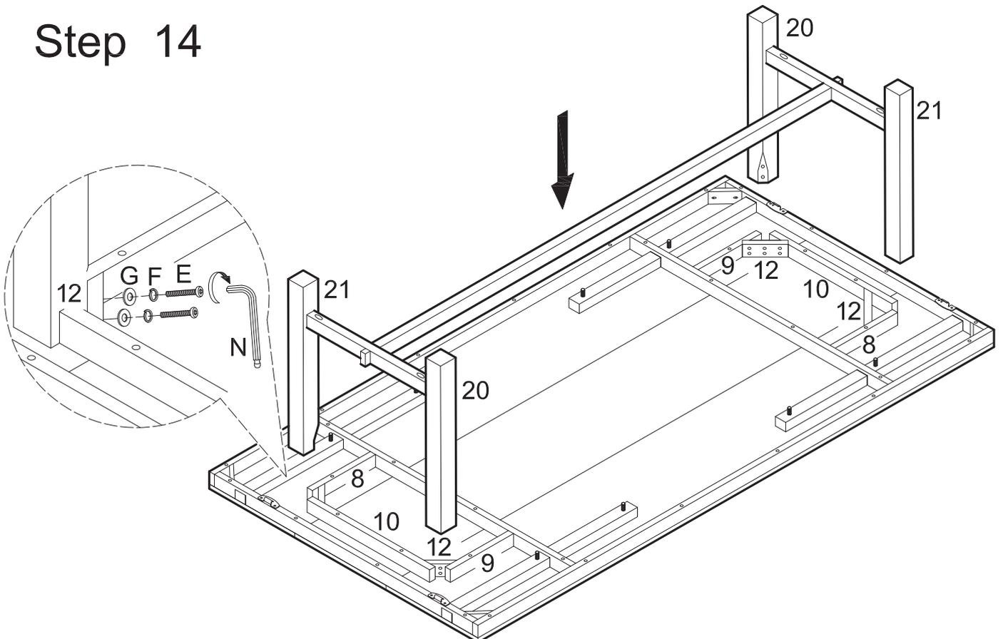
Align legs (20,21) with slats (8,9,10). Attach legs (20,21) to corner blocks (12) using bolts (E), spring washers (F) and washers (G). Tighten all bolts (E) with wrench (N).
