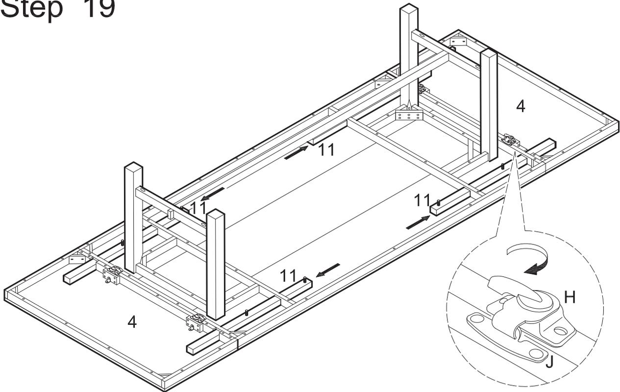
Pull slats (11) through leaves (4). Lock leaves (4) to main table assembly using table lock pieces (H,J).
