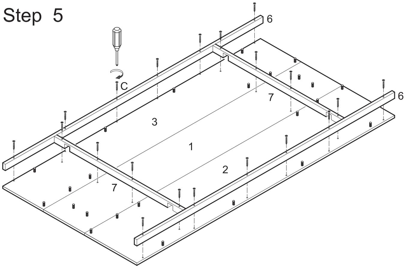
Attach slats (6,7) to table top pieces (1,2,3) using screws (C).
