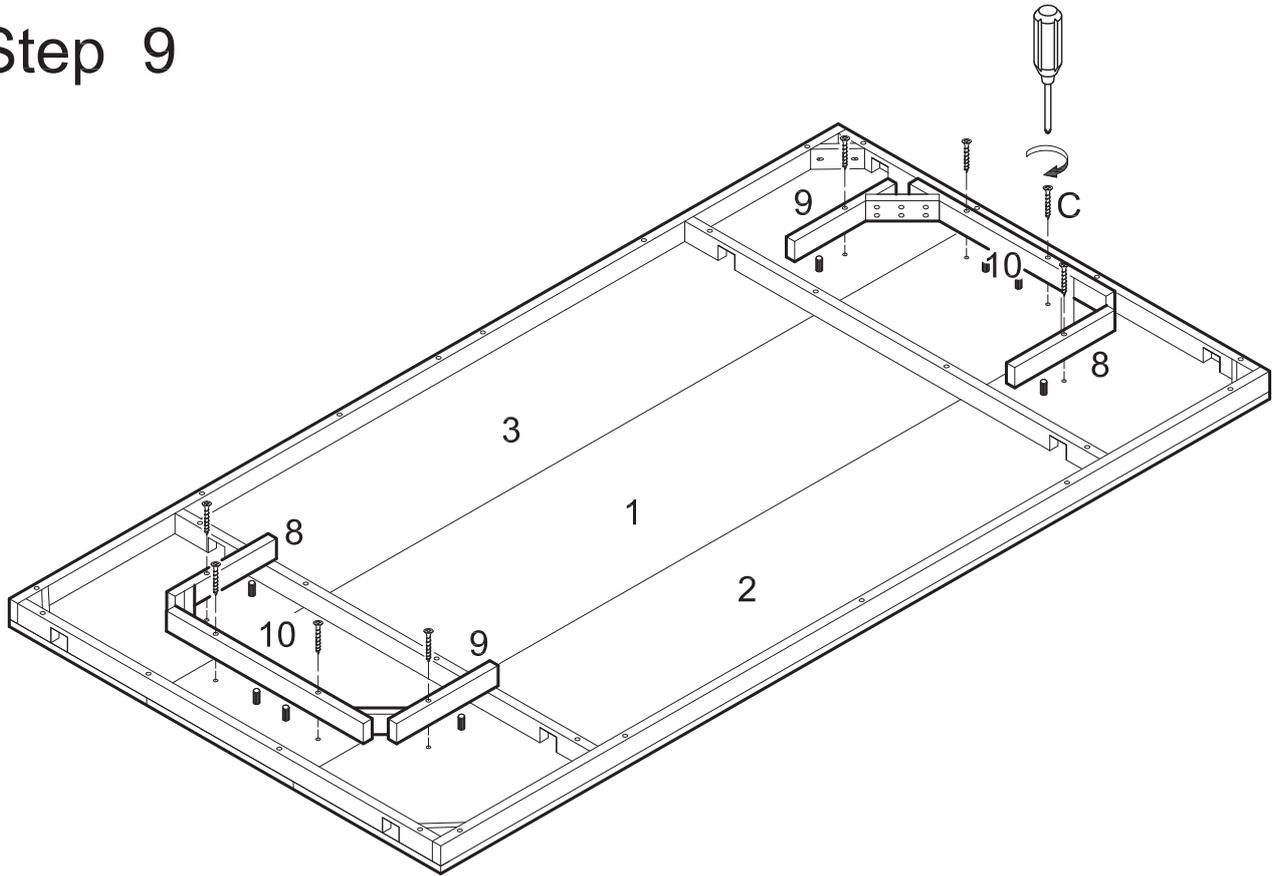
Attach slats (8,9,10) to table top pieces (1,2,3) using screws (C).
