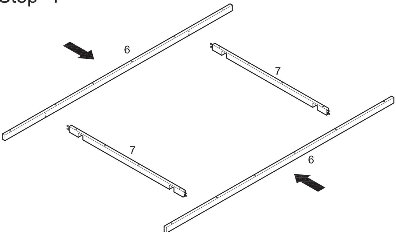
Attach slats (6) to slats (7) using dowels as guides.
