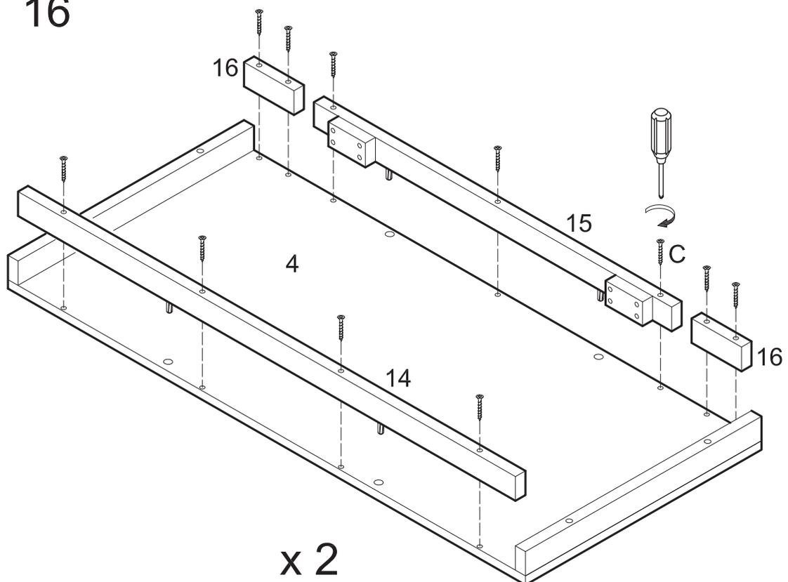
Attach slats (14,15,16) to leaf (4) using screws (C). Repeat this step for second leaf (4).
