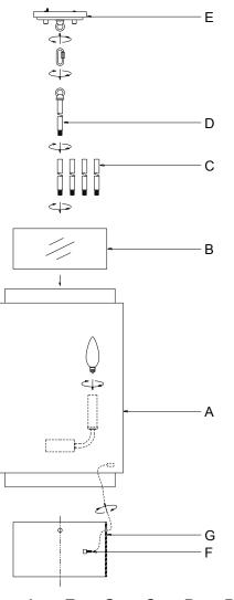
$B \to A \to F \to G \to C \to D \to BULB$
