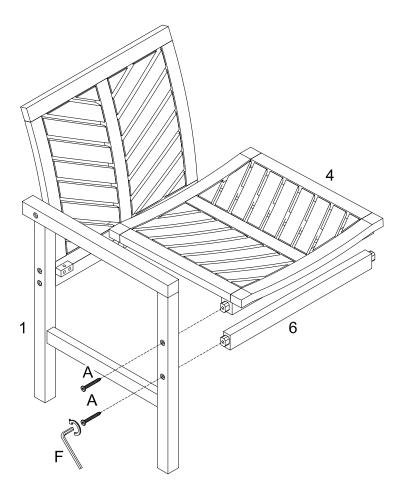
Use bolt (A) and Hex Key (F) to secure part (1) to part (4) and then secure part (1) to part (6).
