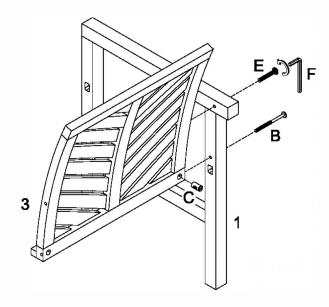
Insert nut (C) into part (3), then using bolts (B,E) and Hex Key (F) secure part (1) to part (3).
