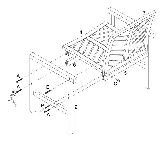
Insert nut (C) into seat panel (3). Then use Hex Key (F) and bolts (A,B,E) to secure part (2) to parts (3,4,5,6).
