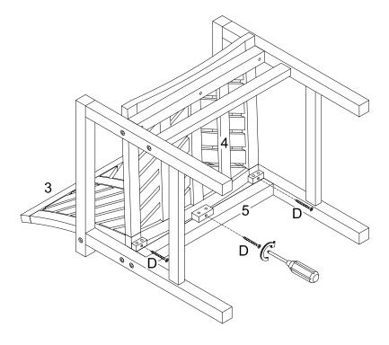
Use screw (D) and a screwdriver to secure seating panel (4) to support bar (5).
