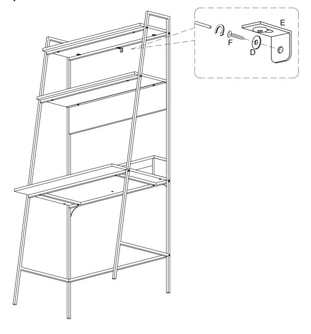
Secure furniture to wall anchor (G) in wall using washer (D) and screw (F) with screwdriver.
