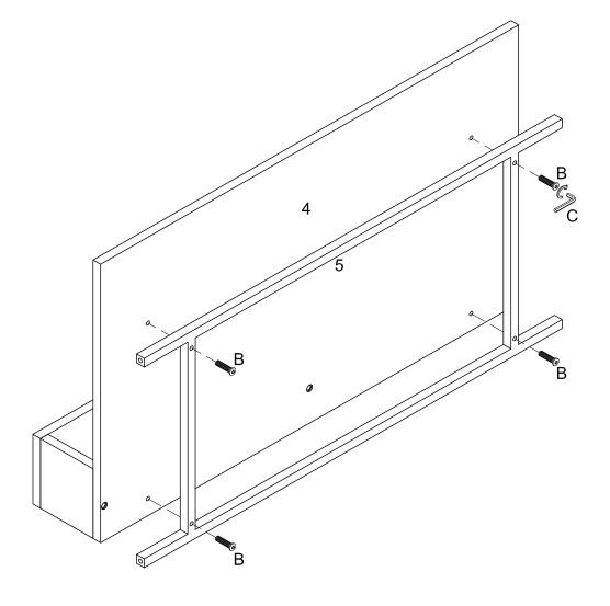
Attach part (5) to part (4) using bolt (B) with hex key (C).
