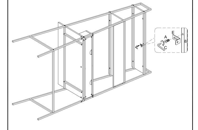
Attach bracket (E) to part (8) using bolt (A) with hex key (C).
