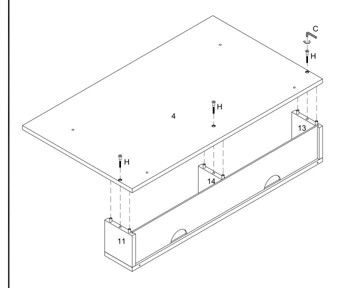
Attach part (4) to part (11,14,13) using bolt (H) with hex key (C).
