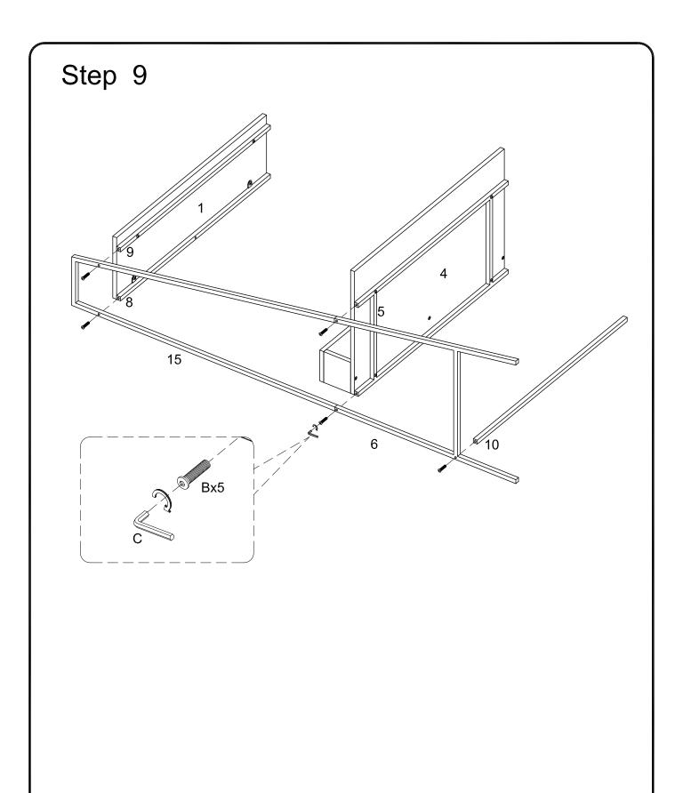
Attach part (15,6) to part (1,9,8), part (5,4), part 10 using bolt (B) with hex key (C).
