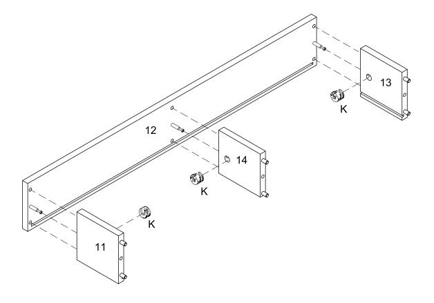
Insert part (11,14,13) to part (12), then secure cam lock (K) to part (11,14,13) with screwdriver.
