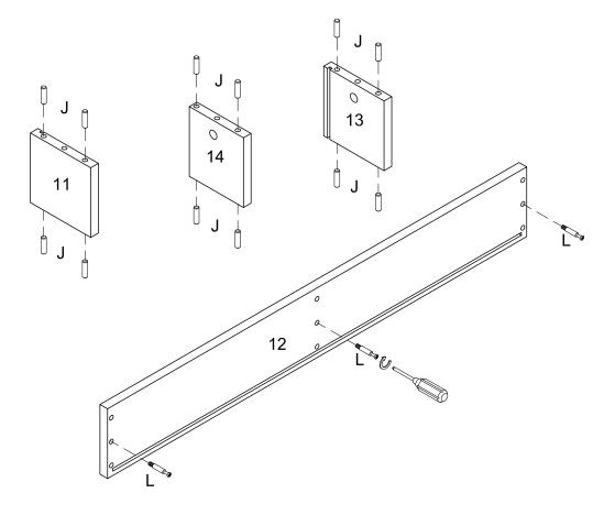
Insert wooden dowel (J) into part (11,13,14), secure cam bolt (L) to part (12) with screwdriver.
