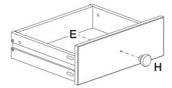
Attach parts (11,12) to part (10), insert panel (13) into groves and secure part (14) with screws(D) Insert knob (H) with screws(E).
