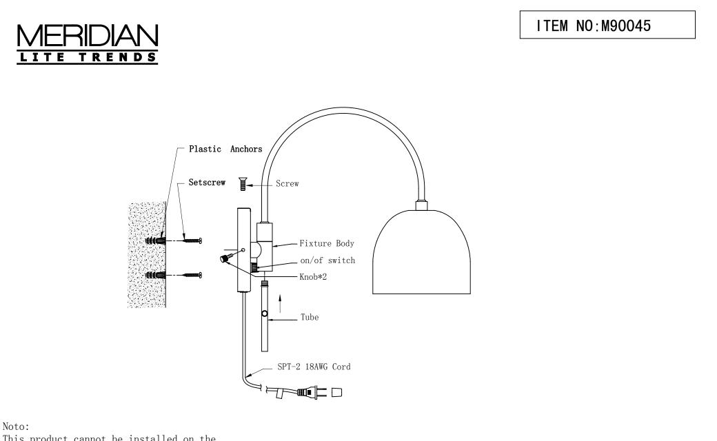
This product cannot be installed on the plasterboard .Advised to install on the wooden board.
