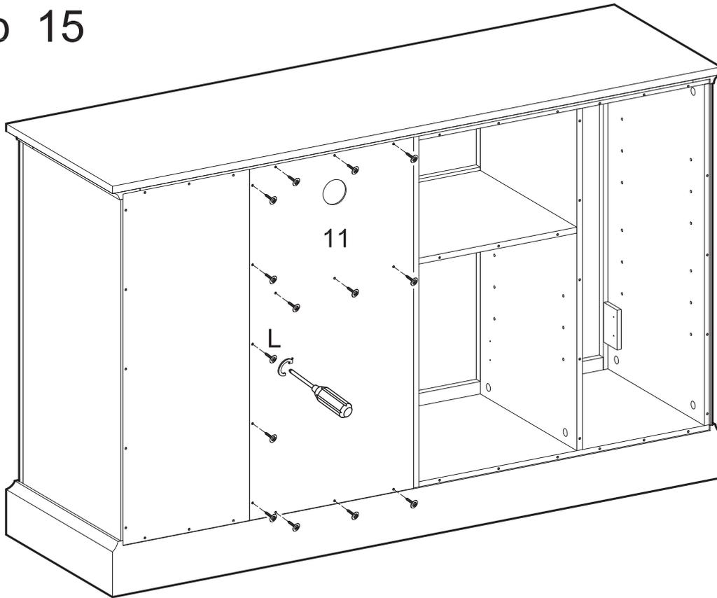
Attach panel (11) to the back of the console using screws (L).
