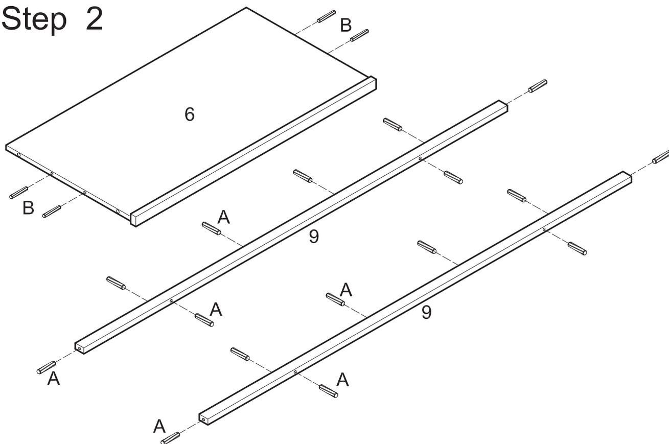
Insert dowels (B) into panel (6). Insert dowels (A) into slats (9).
