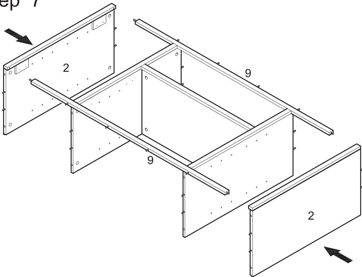
Attach panels (2) to slats (9) using dowels as guides.
