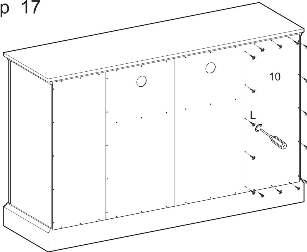
Attach second panel (10) to the back of the console using screws (L).
