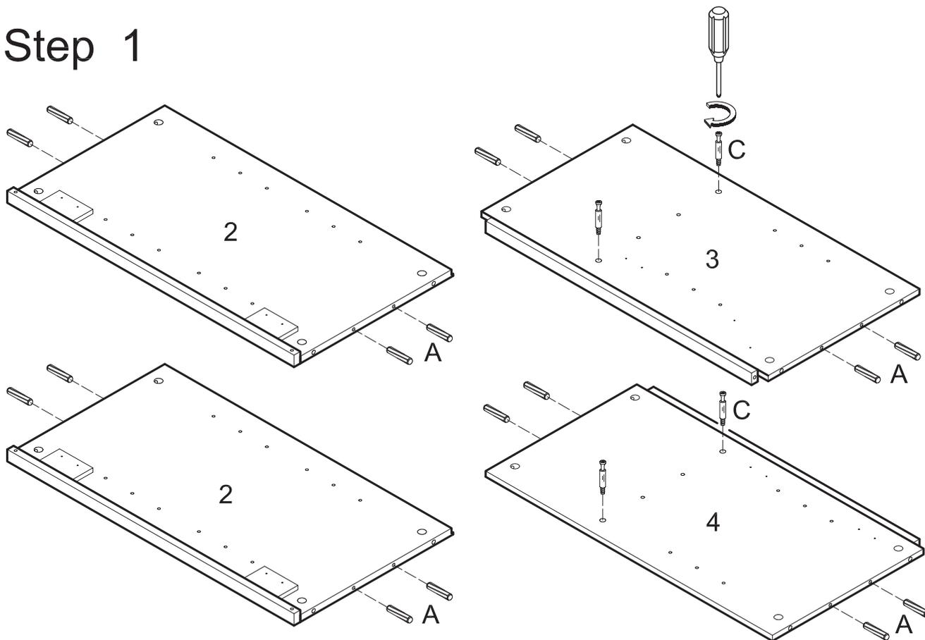
Insert dowels (A) into panels (2,3,4). Screw cam bolts (C) into panels (3,4).
