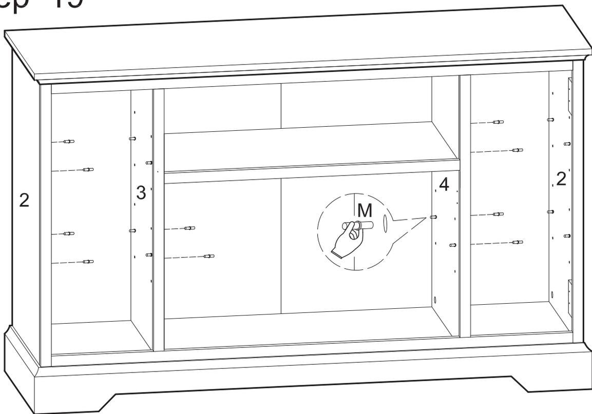
Insert shelf support pins (M) into panels (2,3,4) at desired shelf heights.
