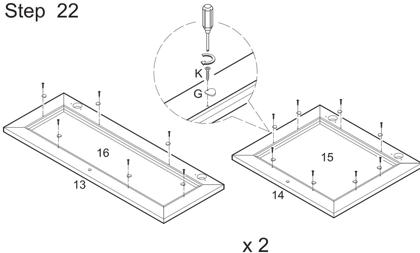
Secure glass pane (16) to door (13) and glass pane (15) to door (14) using metal washers (G) and screws (K). Repeat this step for the second set of glass panes and doors.
