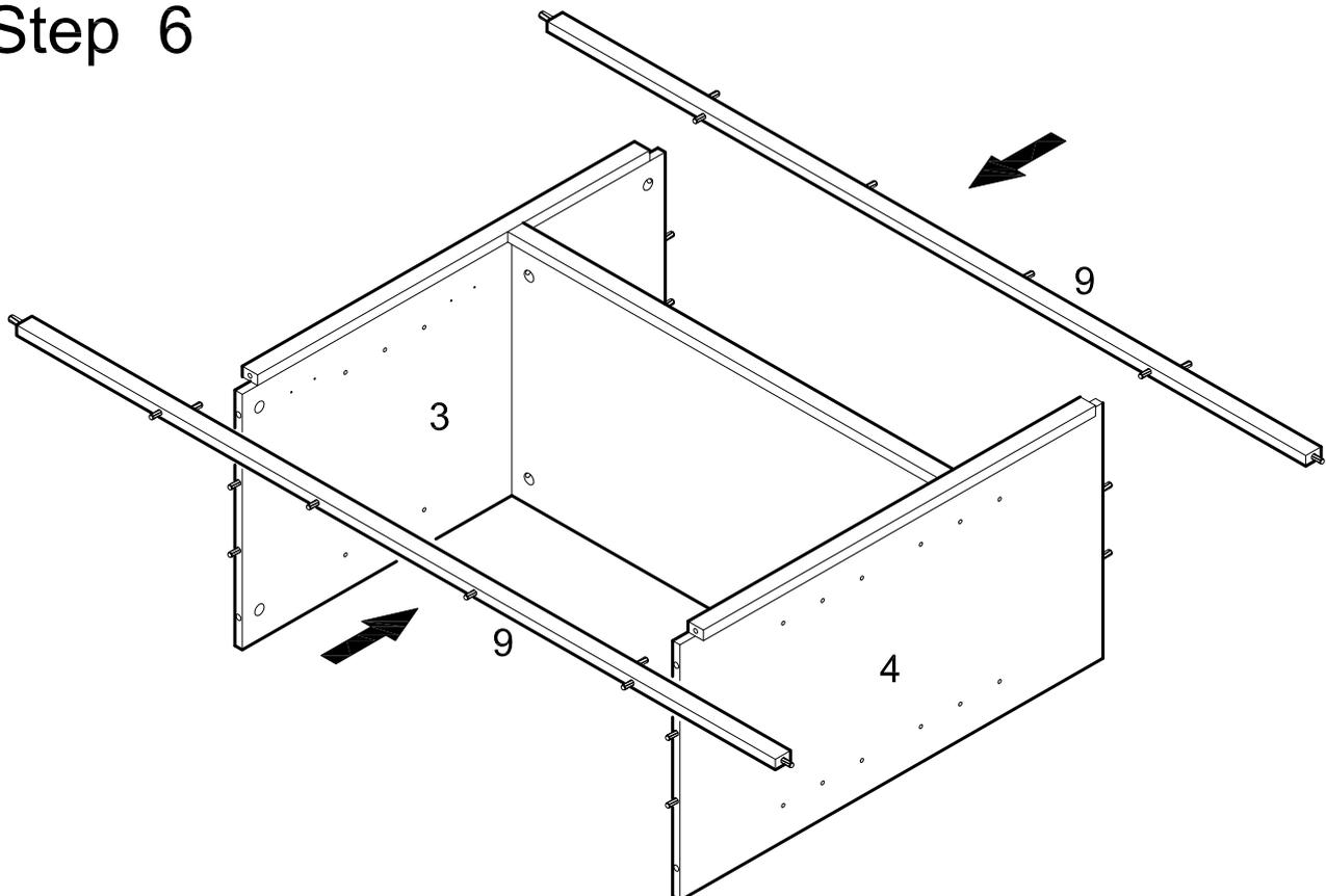
Attach slats (9) to panels (3,4) using cam bolts and dowels as guides.
