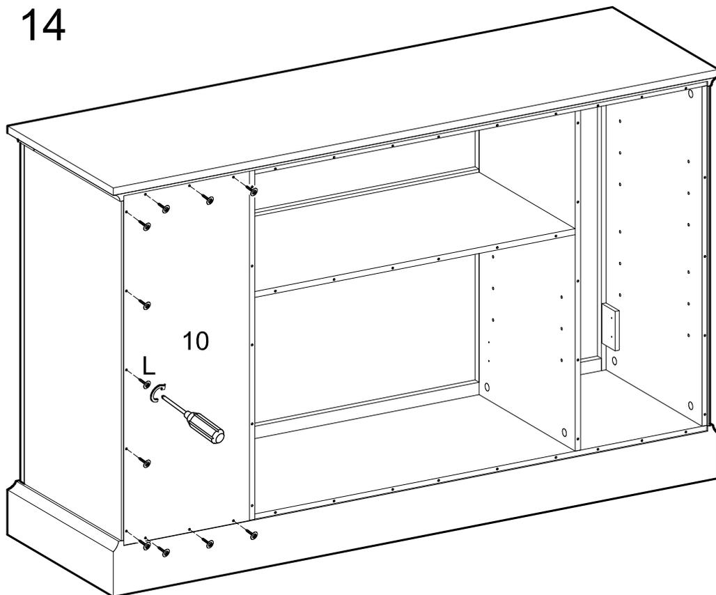
Attach panel (10) to the back of the console using screws (L).
