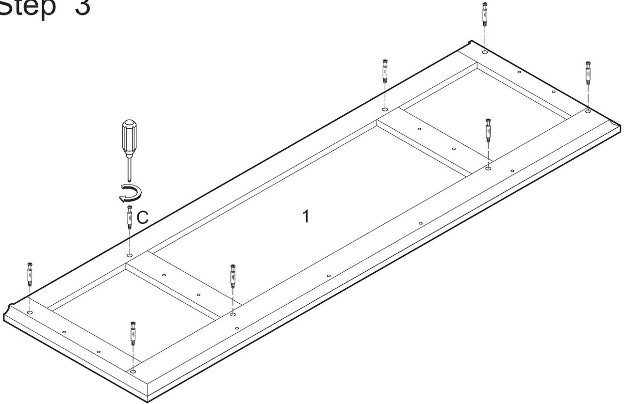
Screw cam bolts (C) into top panel (1).
