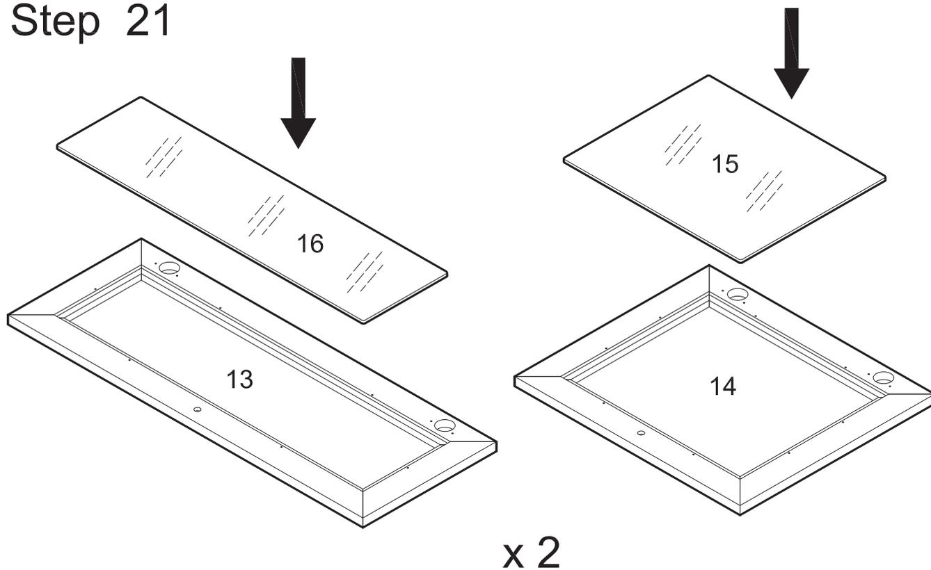
Carefully lay glass pane (16) into door (13) and glass pane (15) into door (14). Repeat this step for the second set of glass panes and doors.
