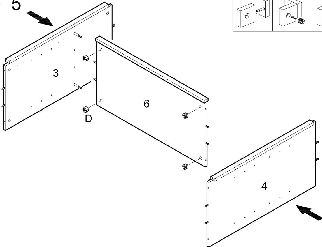
Attach panels (3,4) to panel (6) using cam bolts and dowels as guides. Secure panels (3,4) to panel (6) using cam locks (D). Tighten cam locks (D) with a screwdriver.
