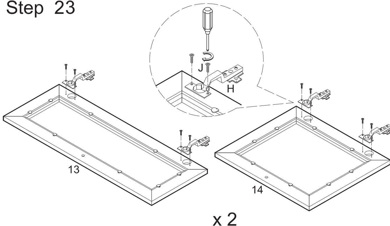
Attach hinges (H) to doors (13,14) using screws (J). Repeat this step for the second set of doors.
