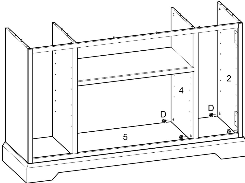
Secure panels (2,4) to bottom panel (5) using cam locks (D). Tighten cam locks (D) with a screwdriver.
