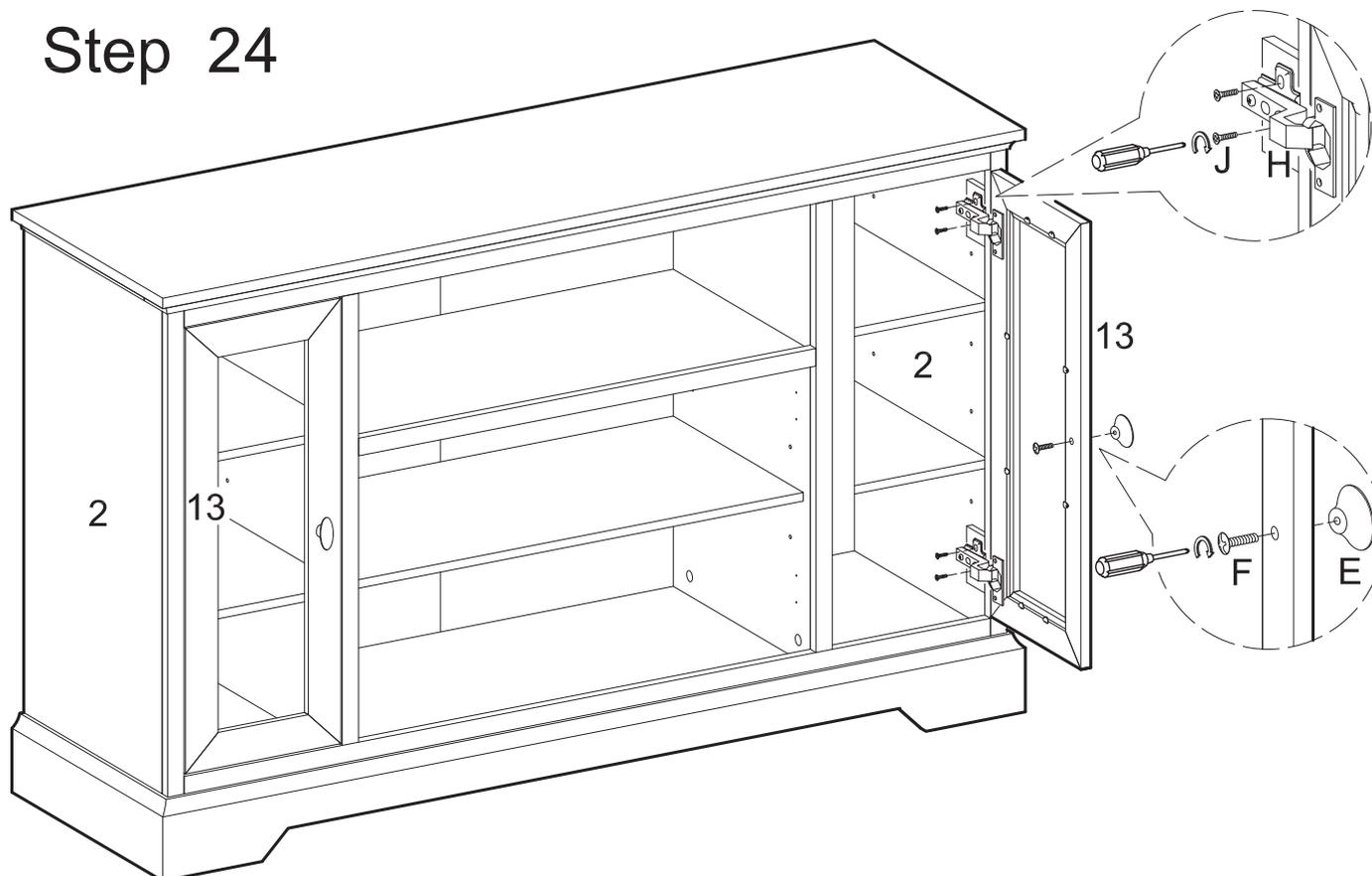
Attach doors (13) to panels (2) using screws (J) at hinges (H). See page 2 for specific instructions on how to adjust hinges so doors are aligned with console as desired. Attach handles (E) to doors (13) using bolts (F).
