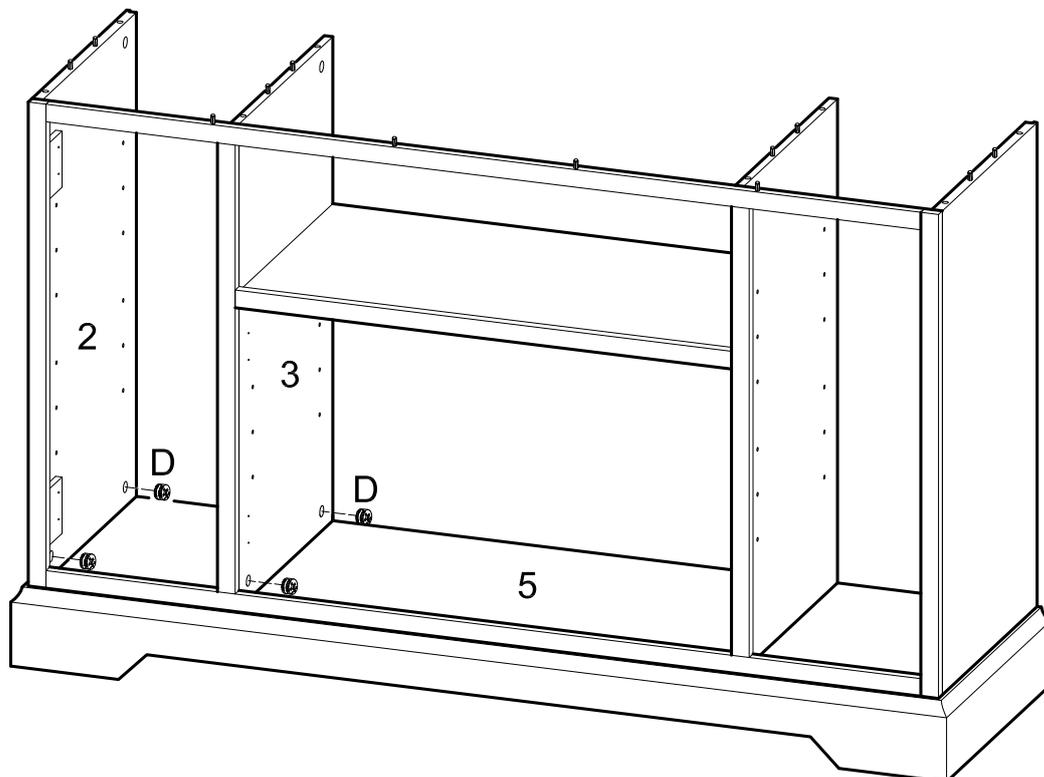
Secure panels (2,3) to bottom panel (5) using cam locks (D). Tighten cam locks (D) with a screwdriver.
