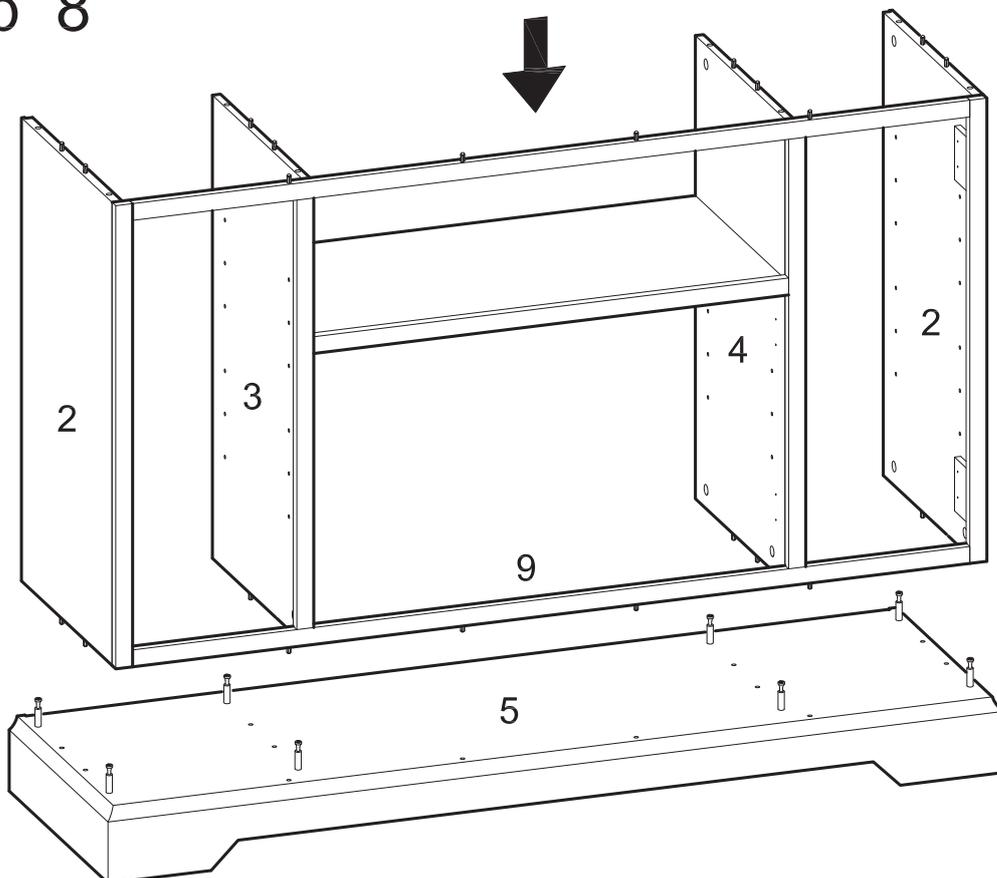
Attach the assembly from the previous step to bottom panel (5) using cam bolts and dowels as guides.
