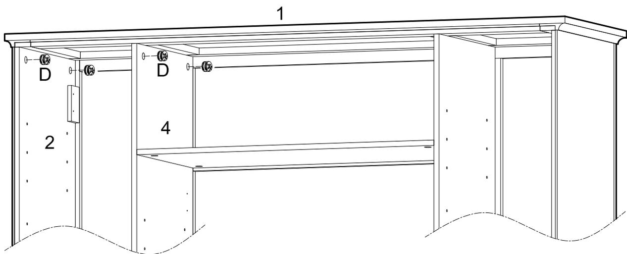
Secure top panel (1) to panels (2,4) using cam locks (D). Tighten cam locks (D) with a screwdriver.
