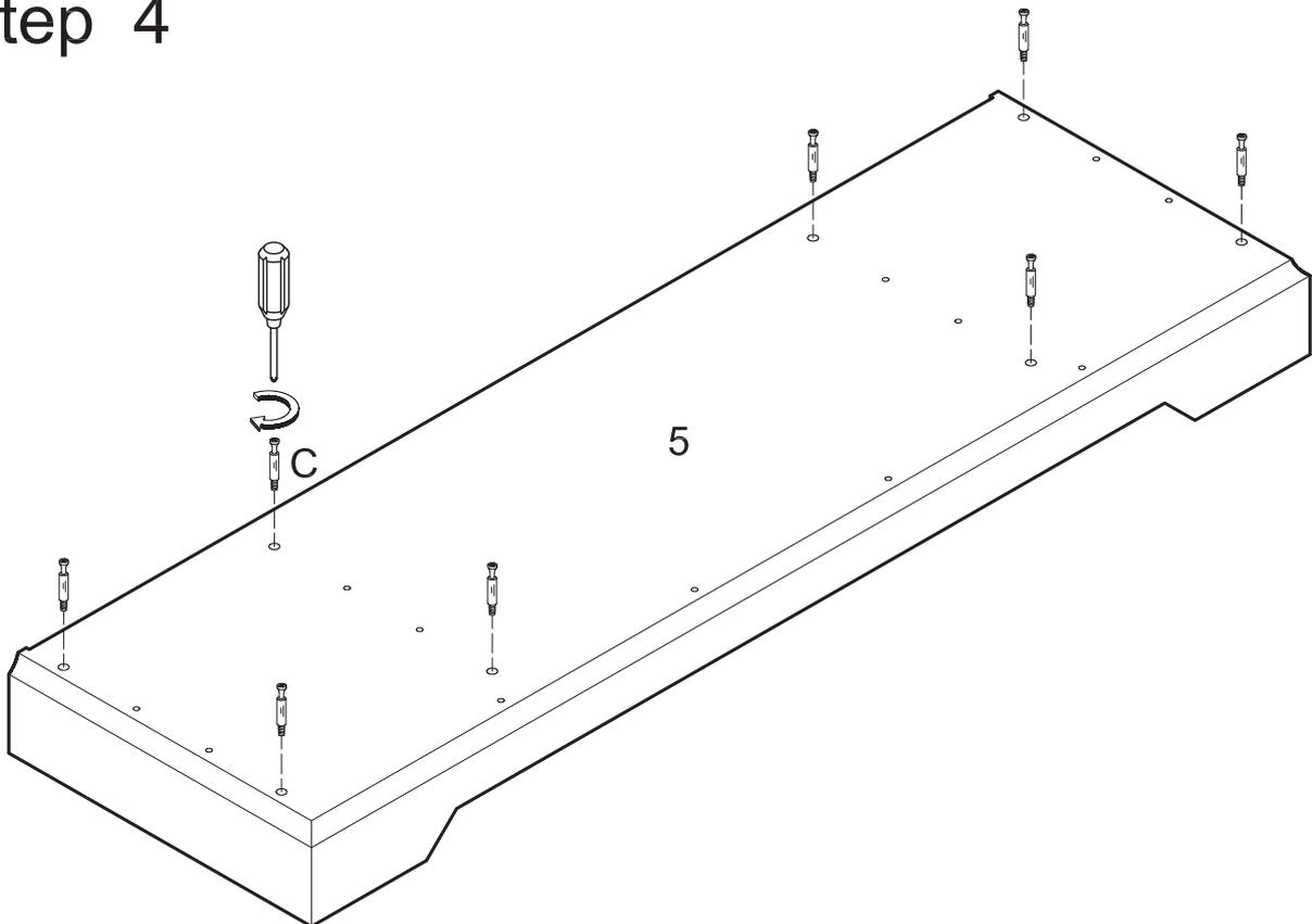
Screw cam bolts (C) into bottom panel (5).
