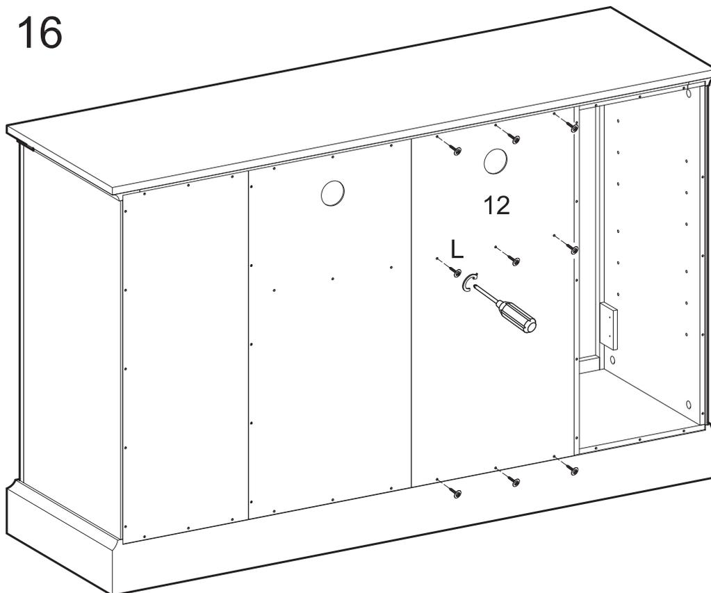
Attach panel (12) to the back of the console using screws (L).
