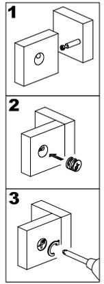
Carefully fit top panel (1) into place using cam bolts and dowels as guides.
