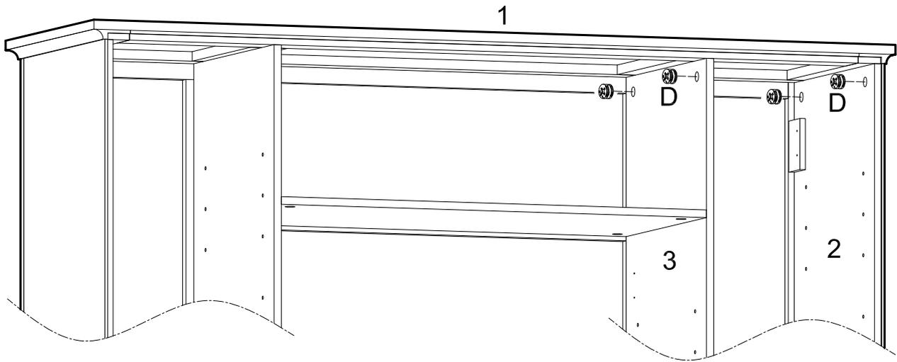
Secure top panel (1) to panels (2,3) using cam locks (D). Tighten cam locks (D) with a screwdriver.
