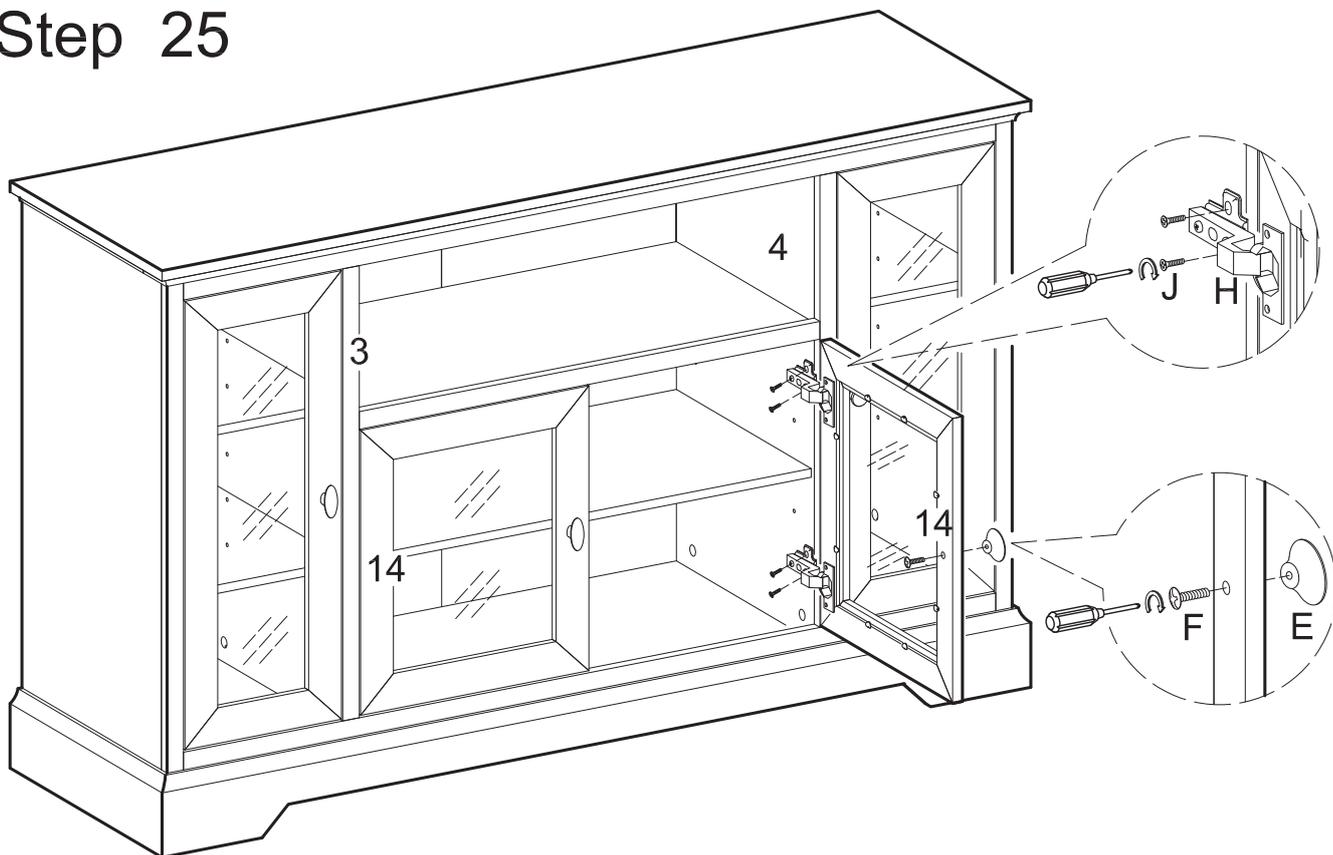
Attach doors (14) to panels (3,4) using screws (J) at hinges (H). See page 2 for specific instructions on how to adjust hinges so doors are aligned with console as desired. Attach handles (E) to doors (14) using bolts (F).
